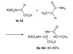
phenylacetylene readily take up acrylamide (within 2–3 h) to give *N*-(1-sulfonylamino-2-polychloroethyl)acrylamides **IIa–IId**. Heating of the reaction mixture to 40–50°C accelerates the process. We observed no formation of poly(acrylamide), though acrylamide is known to readily undergo polymerization in the presence of radical initiators.
